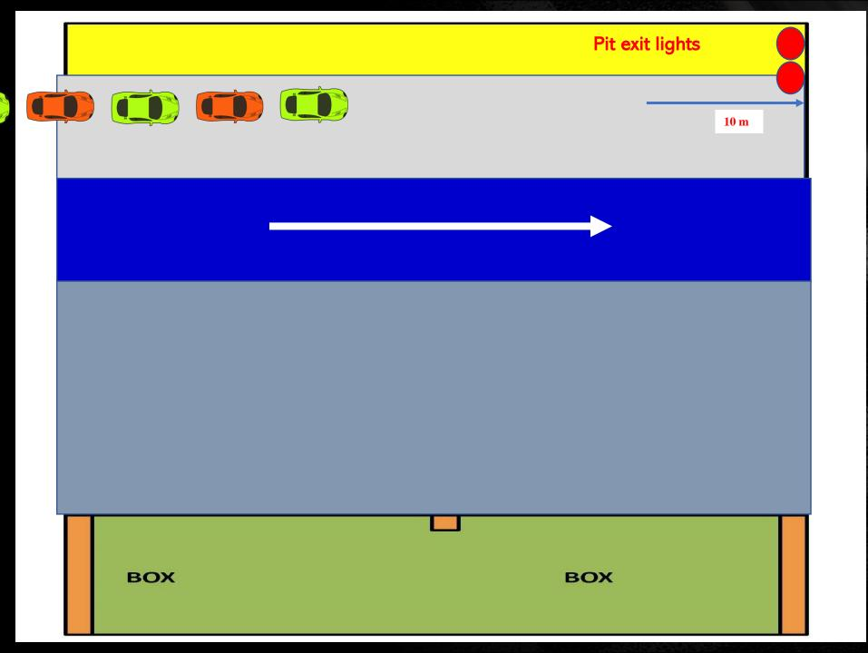
Neutralized track The cars remain in the traffic lane and move towards the pit exit line and stop 10 metres from it
